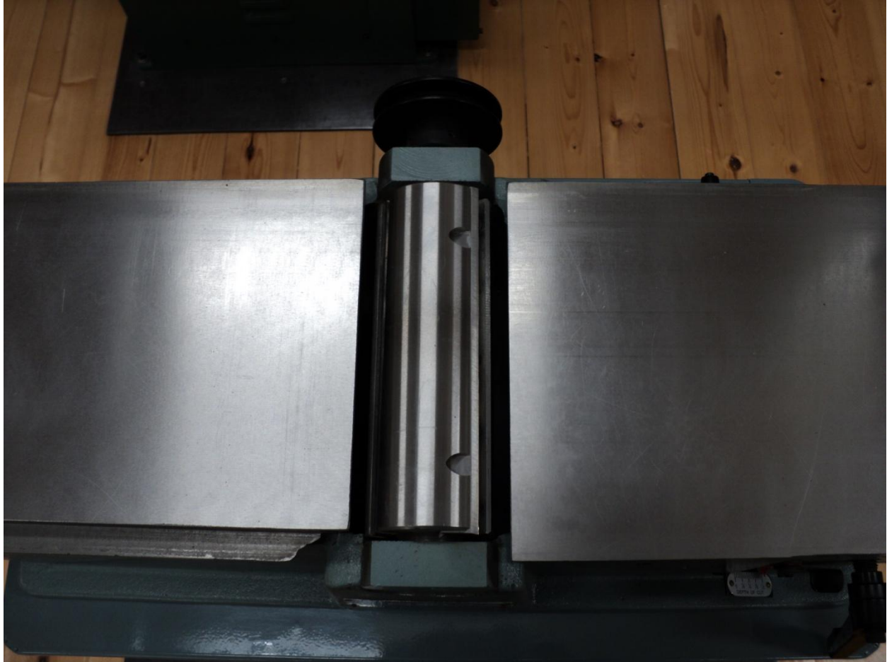
Figure 10 –Jointer with infeed and outfeed tables lowered to allow head removal
