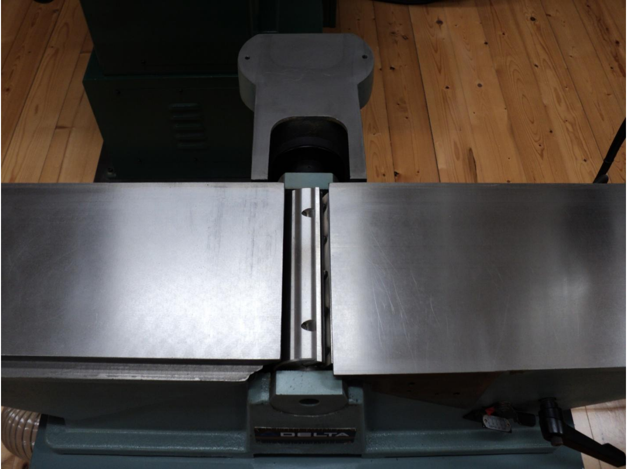
Figure 6 – Jointer after removal of fence positioning bracket
