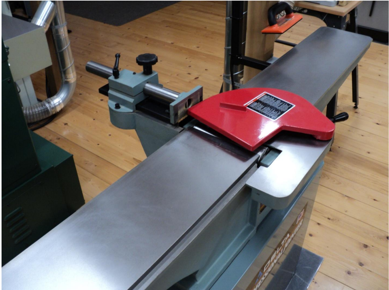
Figure 2 – View of the jointer with the fence assembly removed
