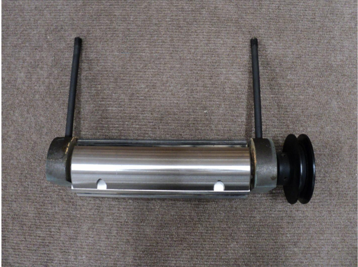
Figure 12 – Knife head assembly after removal from jointer
