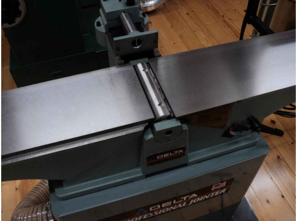
Figure 5 – Jointer after the knife guard support bracket is removed
