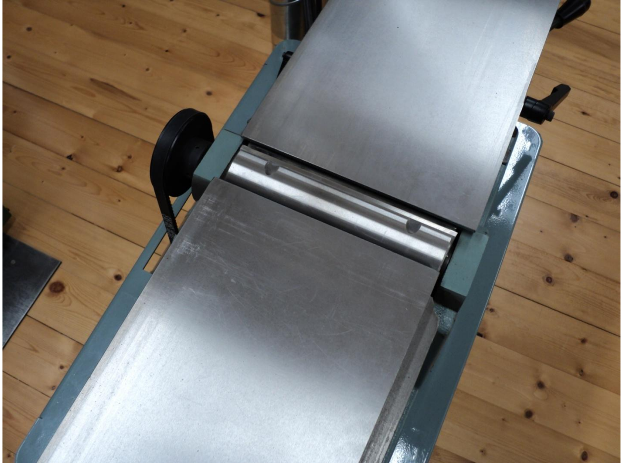
Figure 7 – Jointer after removal of fence support bracket
