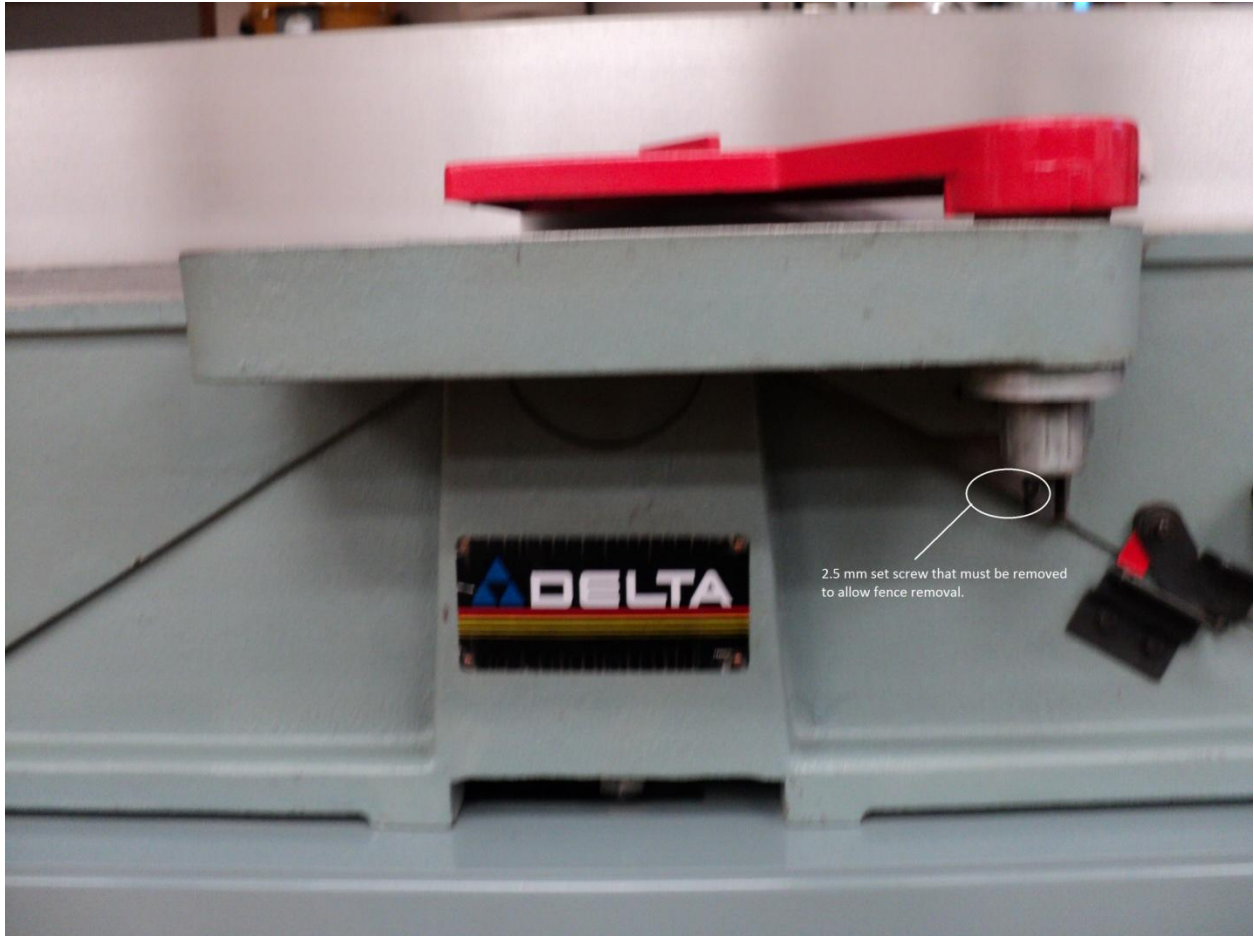
Figure 3 – Front view of jointer knife guard attachment set screw
