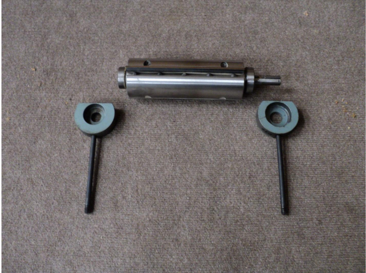
Figure 13 – Knife head with pulley, key, and both bearing supports removed
