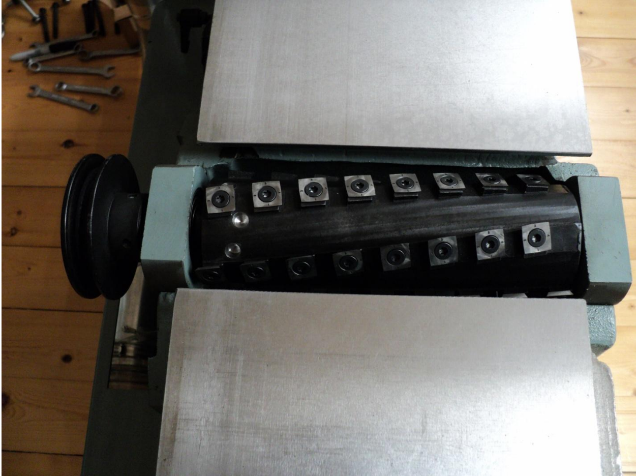
Figure 14 - Shelix® head back in jointer - ready for final reassembly
