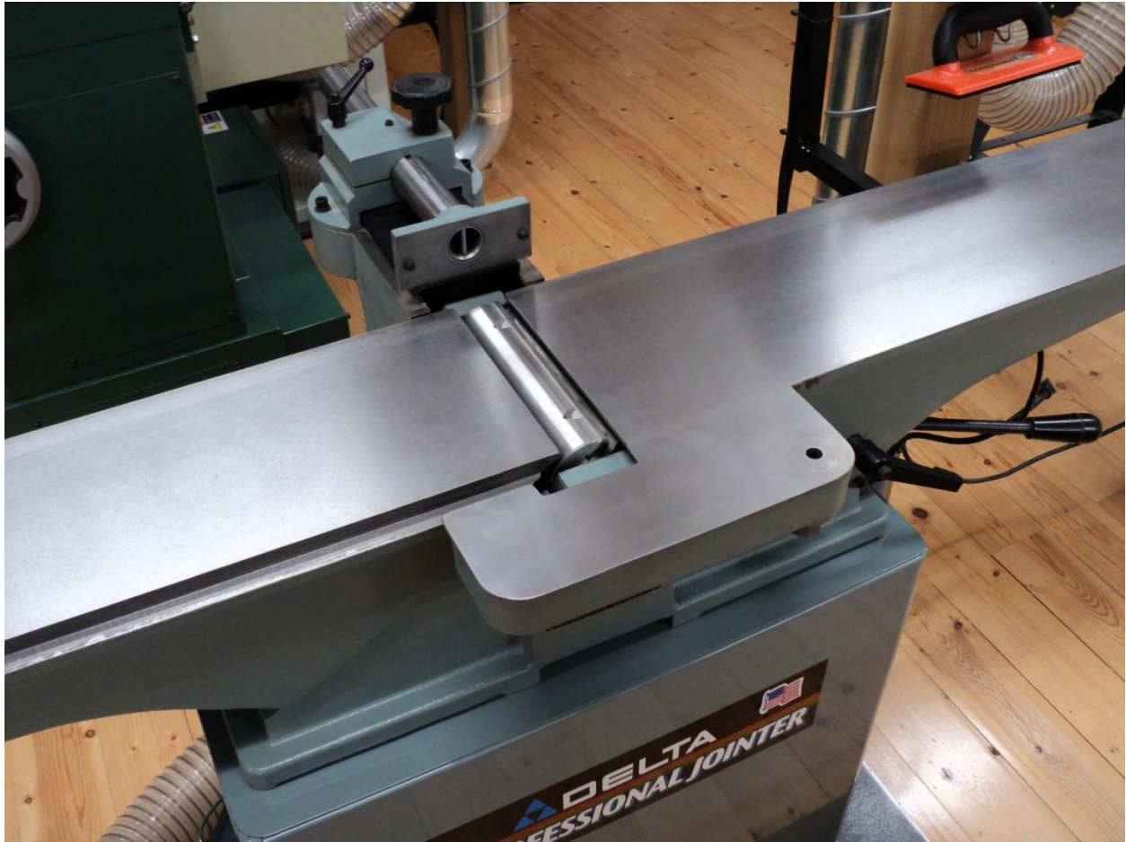
Figure 4 – View of the jointer with the knife guard and fence assembly removed
